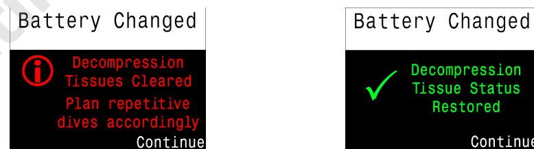
FIGURE 24 After a battery change, you will be notified if the decompression tissues were restored successfully
