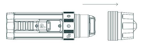
To put the end cap back on, pull back the lock ring on the end cap, and push the end cap back on.
